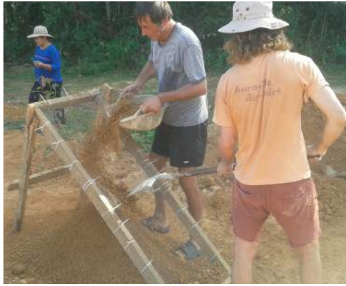
An inclined clay sifter made of 2x4s and plastic mesh. Mesh size of varies depending on the size of clay particles you want
