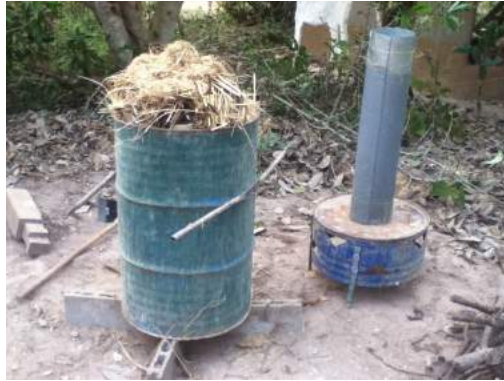
Left: Topping the barrel with kindling after filling with bamboo Right: The bio-char maker in action, reaching 900°C Bio-char maker at Panya Project, Thailand
