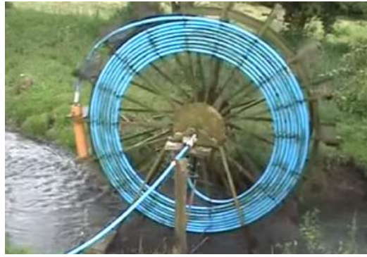
Water wheel uses pvc bent to form a circle
