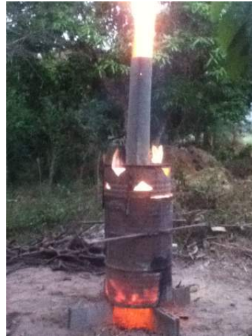
Left: Topping the barrel with kindling after filling with bamboo Right: The bio-char maker in action, reaching 900°C Bio-char maker at Panya Project, Thailand
